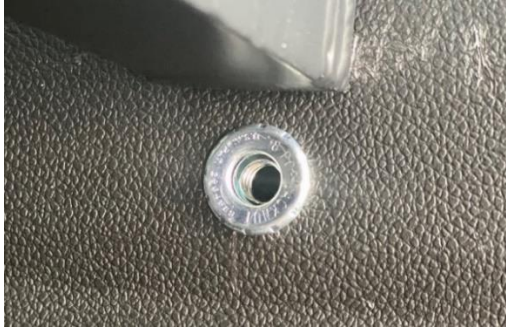
Nutsert fully installed
