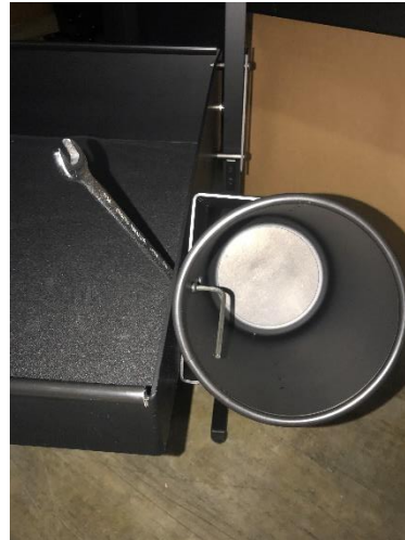
5 - Tighten the cylinder as much as possible with a 7/16 wrench and 4 mm allen wrench (included in kit)
