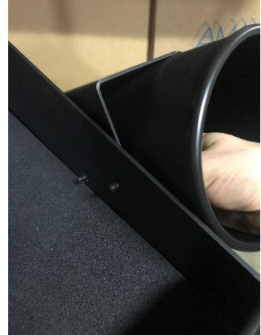
3 - Insert bolts into holes while securing from the inside
