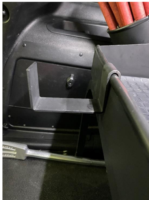
3 – Press down with thumb to the final position as bend goes over the lip of the tray
